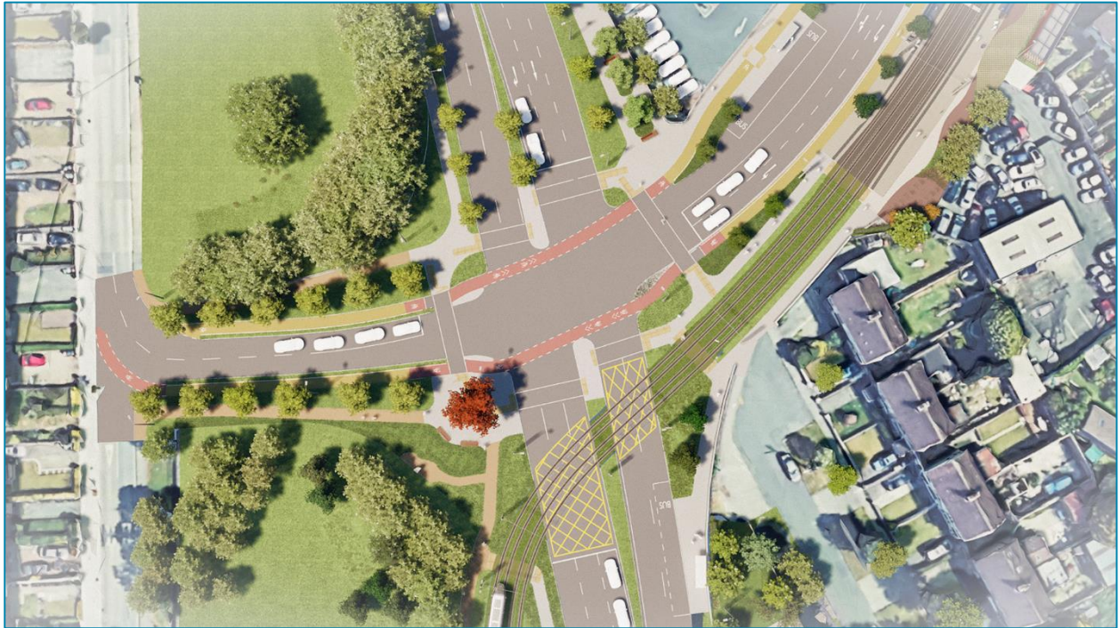
Figure 6-11: Plan of Proposed R135/R104 Junction with new road layout and Luas crossing to south
